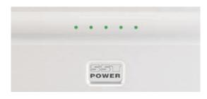
Power LEDs on the front panel indicate each channel's functional status — green for power-on, red for overdrive.
